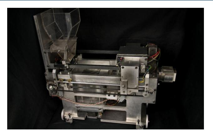
The proposed invention is the first metal additive manufacturing system that autonomously identifies and removes defects during the printing process. More in details, this is a novel Laser Powder Bed Fusion machine equipped with an innovative defect deletion system that combines a subtractive technology (i.e., grinding) and a superficial thermal treatment for in-line defective layer removal driven by intelligent in-situ monitoring methods.
